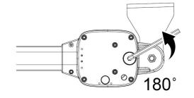
To lock the opener mechanism, insert the hex wrench and turn 180° clockwise.
